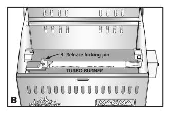
**3.** To remove burner pull locking pin.
