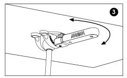
IMPORTANT: Make sure that the handle is tightened fully.
