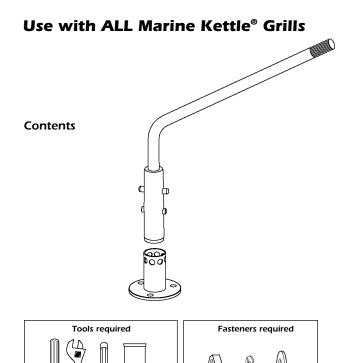
Mount may be installed on any angle horizontal surface. However, in order to use it as a rotating mount, it must be installed in a completely level position. Shims, not provided, may be used during installation to level this mount.
