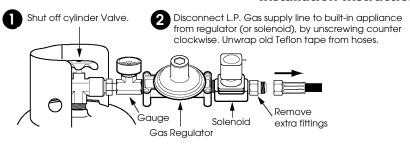
3 Ensure all connections are clean. Connect L.P. Gas Grill Hose Kit between regulator (or solenoid), and L.P. supply line. Wrench tight (clockwise). Remove Female Flare Cap and connect hose (save flare cap).
