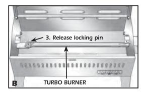
**3.** To remove burner pull locking pin.
