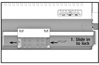
**1.** Slide Grease Tray into either side of the mounting bracket to lock.
