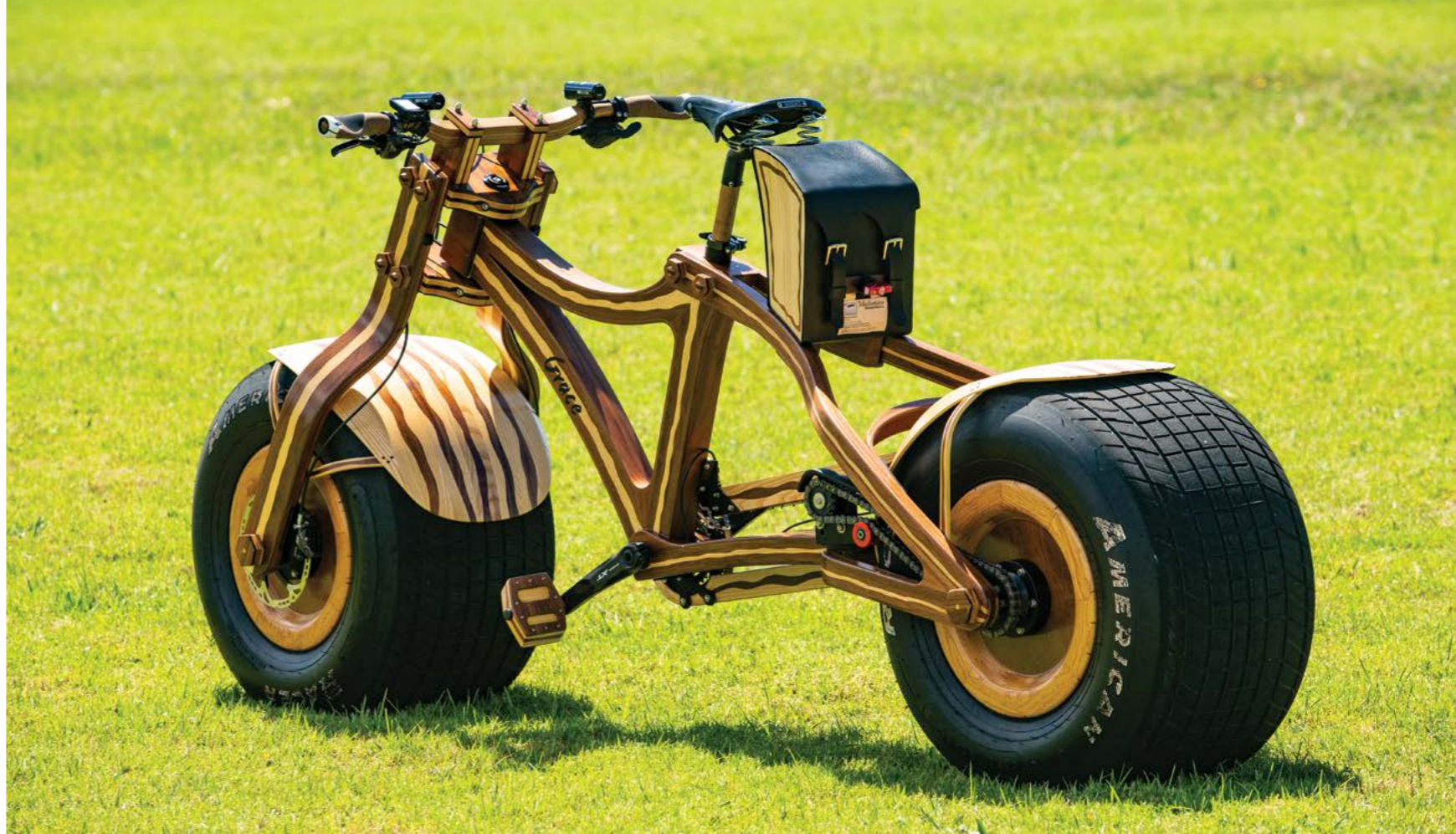
Above: The forks and both sets of stays are laminated to curve around the fat wheels
