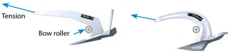
Twin rollers or a large single roller eliminate movement best. This is because two points of contact exist for the anchor instead of just one. If remaining movement is unacceptable, the anchor should be lashed in place.
