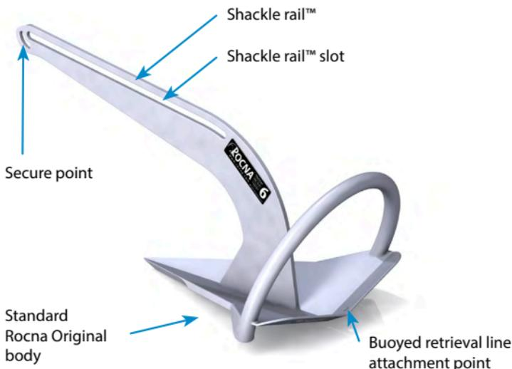
A float shackled to the dedicated retrieval line attachment point at the heel of all Rocna anchor flukes is the ideal recovery system, offering the best chance of a successful recovery in the event of a fouled anchor.
