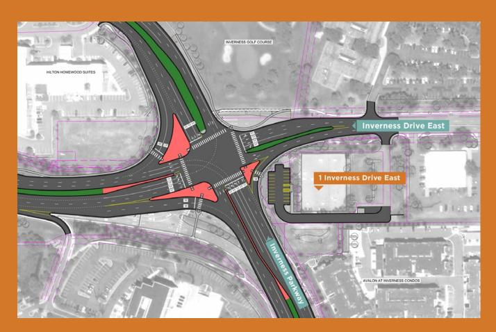
REDESIGN OF TWO EXISTING, CLOSELY-SPACED INTERSECTIONS INTO A SINGLE, TRADITIONAL INTERSECTION TO IMPROVE SAFETY AND MOBILITY.
