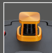
Main LiDAR The main LiDAR sensor array used in mapping and navigation
