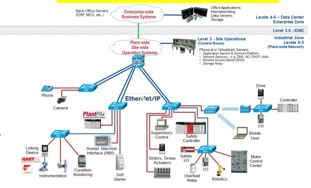
Plant-wide / Site-wide Network Integrated Architecture – Intelligent Motor Control
