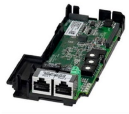
PowerFlex 25-COMM-E2P Dual-Port EtherNet/IP Adapter
