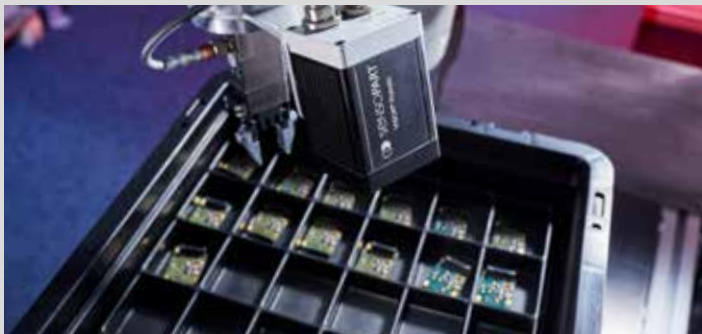
The VISOR® Robotic detects the component's position in a universal tray. It can then be reliably removed. Up to 255 configurations enable utmost production flexibility.
