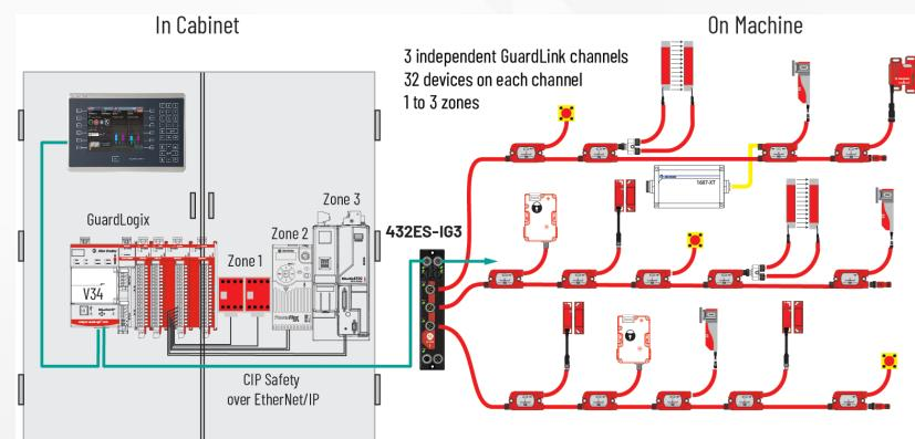
432ES-IG3 located On-Machine™ Taps and safety devices On-Machine™ Three independent GuardLink® channels Up to 32 devices on each channel One to three zones
