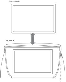
Unzip pouch to install or remove solar panel
