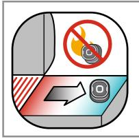
The magnetic base is not designed to withstand high heat and it must be placed on a cool surface. If the surface is too hot to touch, it is too hot for the Kitchen Thermometer mini base!
