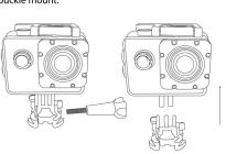
7b. Align the prong on the camera with the spaces on the mount. Push camera into place.
