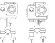
7c. Screw the mounting screw back in to secure the camera to the moun
