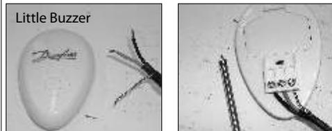
The resistance should be measured between the two conductors, blue and black. Compare the measured resistance to the resistance listed on the product label (on the power lead). Also, measure the resistance between the blue, black and shielding/ground wire. Both should read infinity. Record the resistance on your warranty card.
