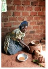
In Uganda, villagers are learning how to build *rollena* stoves out of clay. The stoves use less wood, cook faster and produce less smoke. They are also portable.
