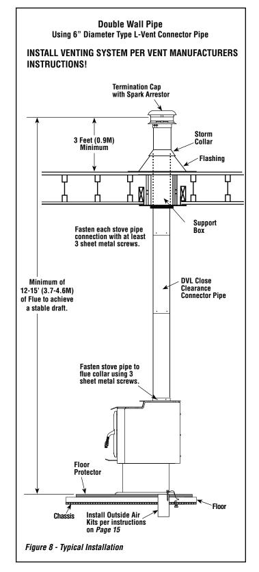
Chimney Connector Systems and Clearances from Combustible Walls for Residential Heating Appliances (NFPA 211) Refer to Figure 9.
