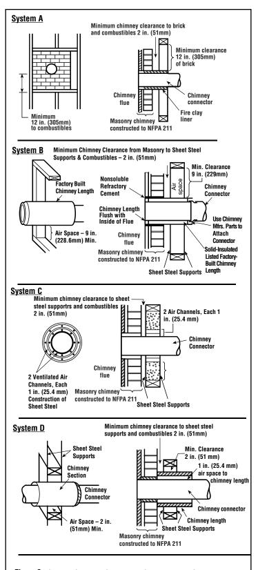
Figure 9 - Chimney Connector Systems and Clearances from Combustible Walls
