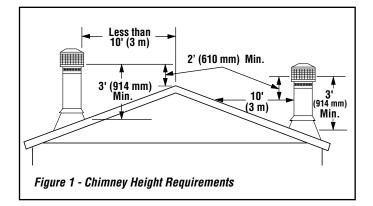
To pass inspection in nearly any jurisdiction, the chimney must meet both safety and exhaust flow requirements. The (3' by) 2' by 10' rule applies to both masonry and factory-built chimneys.
