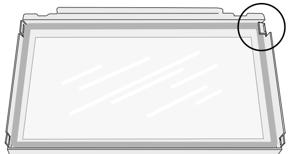
Figure 41. Bend the retainer tabs back enough to release the glass panel.
