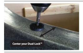
**3.** Place your cover over the well. Use a marker to mark the location of the Dual-Lock™ disc. You will use this mark to attach the corresponding Dual-Lock pad to the underside of your cover. Clean the area under the cover before you adhere the Dual-Lock Pads.
