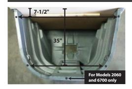
**1.** You will be installing 4 or 5 Dual-Lock<sup>™</sup> discs to your well based on model. Models 2060 and 6700 have 5 anchor points and model 2062 has four.
