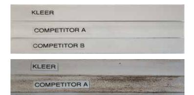
Results from a dirt intrusion test show how much easier Kleer is cleaned compared to competitors.
