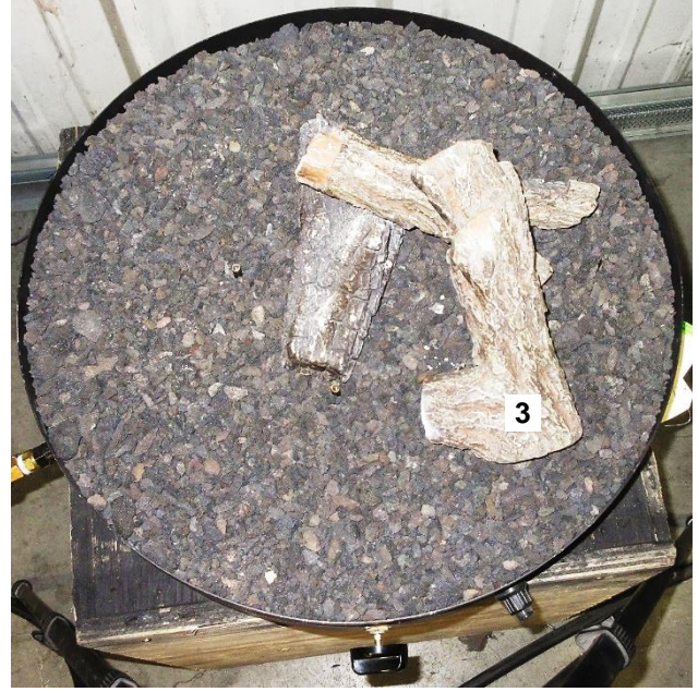
Place Log 3 on top of Log 2 as shown
