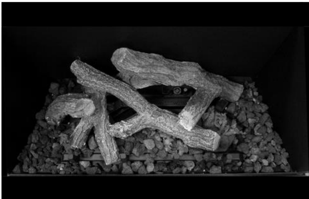
STEP 5: Fill in the rest of the burner pan and ember plates with lava rock. Do not place lava rock on any of the burner ports.
