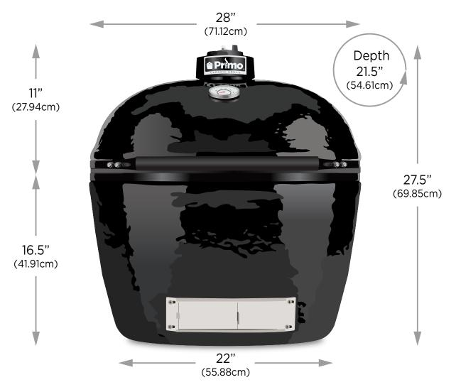
12" (30.48cm) of clearance is required behind the grill to open properly. A minimum of 2" (5.08cm) of clearance is required around the exterior surface of the grill.
