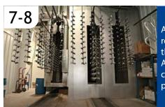
A 200 MPH air blast removes water drops from the pre-treated aluminum. A convection oven completes the dry-off process.
