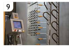
Powder is applied with 18 automated and 2 manual spray guns. Compressed process air is dried to -35°F Dew Point for superior adhesion.
