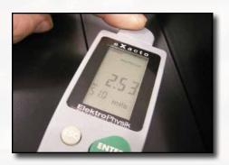
Coating Thickness Test
