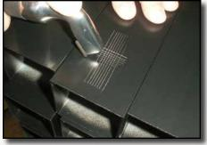
ASTM D3359 Crosshatch Test
