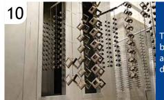
The powder coating is then bonded and adhered to the aluminum substrate in a 400 degree cure stage.
