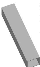
**Step 1:** Measure the opening height. Cut the column 1/8" shorter than your measurement. Cut the column to the desired length with a fine-tooth carbide blade
