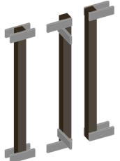
Step 5: Fit the L-Shape cap and base around the column. Secure the cap and base with a finish nail gun or galvanized or stainless steel trim screws
