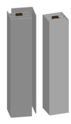
Step 4: Apply a continuous 1/4" bead of urethane adhesive caulk (included) along both mitered edges of the column half. Use a pneumatic finish nail gun to fasten the two halves every 6-8" along both sides of the column.
