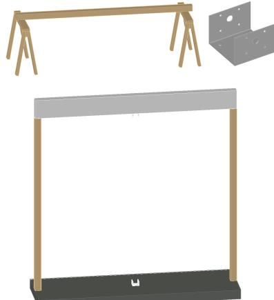
**Step 2**: Use code-approved fasteners and install post mounting brackets (supplied by others) to the beam and floor. Use a plumb bob or level to ensure brackets are aligned and plumb both front-to-back and side-to-side.
