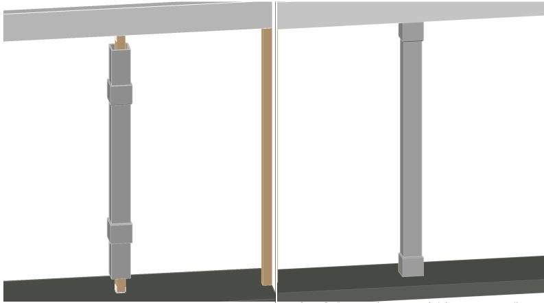
**Step 7**: Use a jack or wooden post to raise the beam approximately  $\frac{1}{2}$ " to install the SmartColumn  $^{\text{TM}}$  into the post mount brackets. Remove the temporary bracing and allow for the beam to slowly come to rest on top of the structural post. Use code-approved fasteners to connect the structural post to the post mounting brackets.
