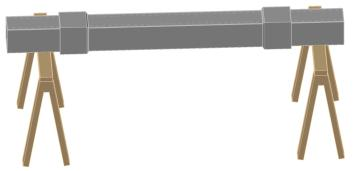
**Step 4**: Once the shaft is cut to length, locate the center of the shaft and make a mark. Measure down 1-1/2" from the center mark at each end of the shaft and make a mark.
