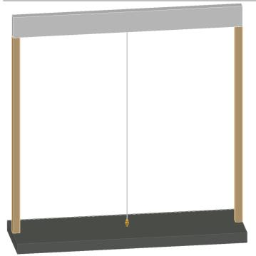
**Step 1**: Insert temporary braces to support the beam at its final finished height. Measure the clear span distance between the floor and bottom side of beam and make note of it. This will be the OVERALL height of the pressure treated structural post inside your SmartColumn $^{\text{TM}}$ . Cut the post to the overall height dimension minus the thickness of the 2 post mounting brackets.
