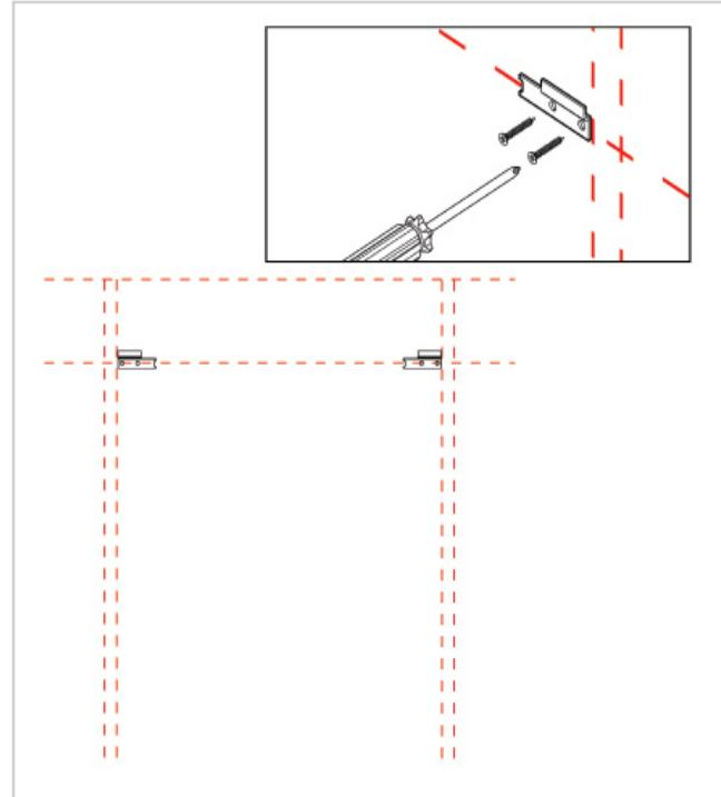
In order for to complete the steps below the red screw found on the wall unit on the hanging bracket will need to be screwed all the way out.
