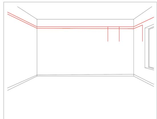
Draw a vertical line **20mm** inside either side of the pre marked wall unit positions.
