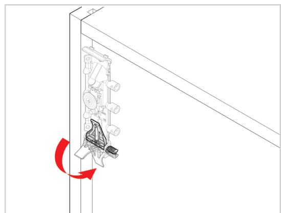
Secure with provided **2x20mm** screws per bracket.
