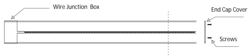
1. Remove the end cap cover, cut to the appropriate size as required, then install the end cap cover back on the track.
