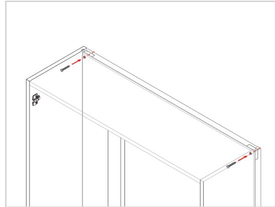
**Before attaching the units together, ensure that the Linea / Milano profile cutout of both units align.**
