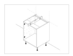
Screws and fixings for attaching the cabinet to the wall are not provided, as these vary depending on the wall material and construction. Check that the appropriate fixings for the wall construction are used.
