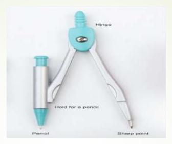
The two legs of the compass are joined at the hinge. Make sure that the metal pin at the hinge is fitted tightly so that the two legs of the compass will not open too easily. Also make sure that your pencil is sharpened. A blunt pencil will lead to diagrams that are not accurate.
