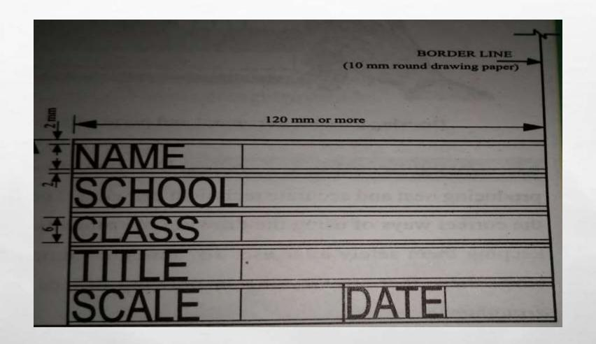
Border lines are drawn on paper in order to obtain margins with visible lines. Usually drawn all round the four sides of the drawing paper. Border line dimension is usually 10mm from the edges of the drawing paper.
