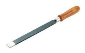
2. Half round scraper: Also called 'bearing scrapers, as they're used for scraping the inside of bearings and other curved surfaces to achieve a better mating surface, curved blade scrapers have two sharp edges.
