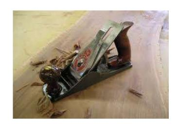
ii. **Fore plane:** Like the jack plane, it is used for roughing out wood and for straight planning.
