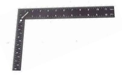
**o Try-square:** The try-square is used for testing the squareness of a surface at 90 degree.
