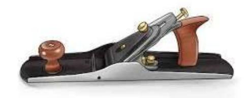
iii. Smoothing plane: This plane is the smaller version of the fore plane. It is used for smoothing the surface of wood after the jack plane has been used.
