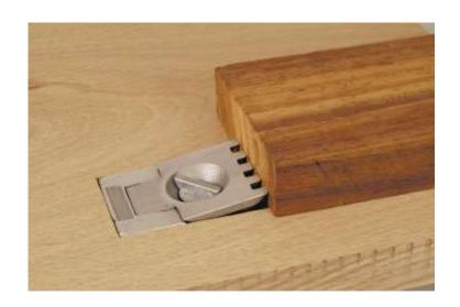
d. **Bench hook:** Bench hook is used to provide a stop against a piece of wood being worked by holding steadily while cutting, planning, or chiseling that piece of wood
