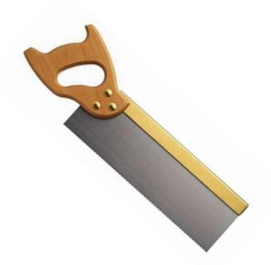
ii. Dovetail saw: This is similar to but smaller than tenon saw, it is used to cut dovetail joints and other simple jobs on the bench.
