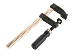
g. Sash Clamp: It is used for wider and bigger jobs for assembling and gluing operations. They vary in size and are normally used in pairs. The slides are arranged on either side and scrap wood is placed between each face and the work. This protect the work when the thread is tightened.
