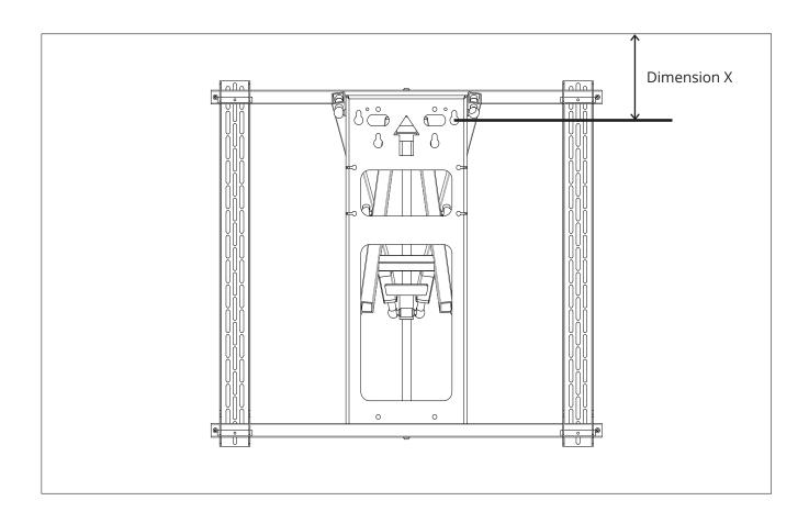
Offer the PS Bracket up to the back of the screen, lining up the screen's VESA holes with the corresponding slots on the PS Bracket Screen Mount. Measure from the top of the screen, down to the top mounting hole on the Wall Plate (Dimension X as indicated above) to determine positioning of the top wall fixing holes.
