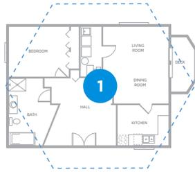
4. Before moving WAP 1 to measure the location for WAP 2, use the WiFi analyzer to test the RSSI value multiple times around WAP 1, ensuring the RSSI value does not drop below -70 dBm.
