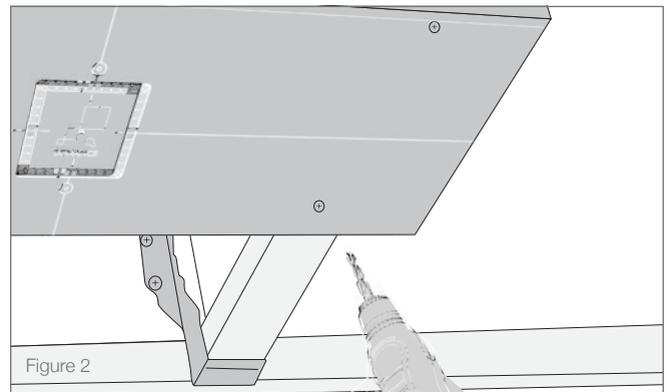
**NOTE: BE SURE TO LOCATE THE TL MOUNTING PLATFORM 15" FROM THE FRONT EDGE OF THE BPS6 TL FROM THE CENTER OF THE MOUNTING PLATFORM CONNECTOR.**
