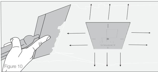
5. Continue to build coats three and four in a similar fashion. Build upon the previous layer and expanding the mud perimeter over the previous layer's perimeter. On the 4th and final coat, be sure to completely cover the sanding shield with mud as demonstrated above. Allow this coat to dry. This will be the last and final coat before sanding. (see Figure 12).
