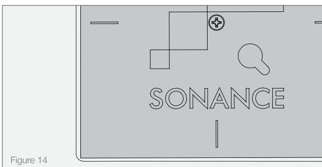
3. Once the sanding is complete, push firmly on the sanding shield to break any adhesion to surrounding surfaces. Next, remove the screw in the center of the shield. Then remove the shield using a screw and a pair of pliers or a slotted screw driver (see Figure 15).
