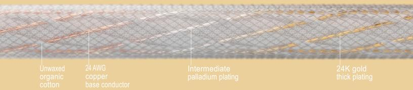
NAKED interconnects start life as a solid-core copper conductor of the utmost purity achievable. We then anneal the conductor surface in hydrogen-rich environment for maximum conductivity and purity before plating with palladium. This is followed by a thick, 24K gold plating. The gold is conductive while preventing oxidation of the copper conductor. The palladium slows down the diffusion of the copper into the gold.
