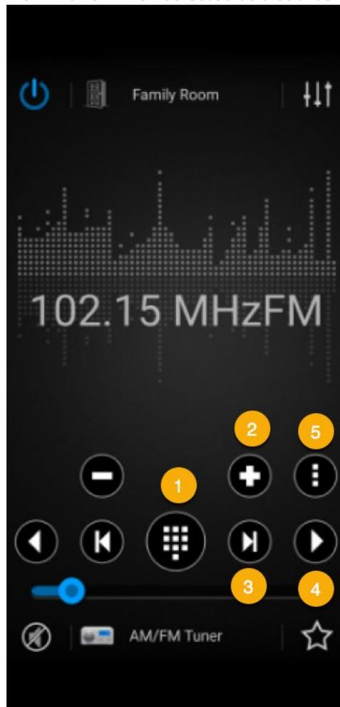
1. Dial pad: This expands the dial pad allowing you to enter a specific frequency and toggle between AM/FM.
