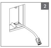
For retrofit installation, locate an existing low-voltage electrical box. For new construction, choose a location for a electrical box. The PoE Splitter can be used with US, UK and Euro single gang electrical boxes. NOTE: The Surface Mount can be installed in portrait or landscape orientation with a single gang electrical box.
