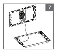
Connect the appropriate power source identified in the Power and Wiring Guide (found in (f) PoE splitter box). Place PoE splitter into the single gang box located in the wall with the iPort logo facing out.
