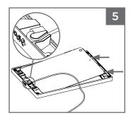
Plug in the lightning to USB cable into the iPad and lower the iPad face down into the bezel with the cable on the left hand side. Carefully wrap the iPad cable around the metal loop located on the (a) bezel. To lock the iPad in place, deploy the second and third toggle located on the right side of the Surface Mount (a) bezel.
