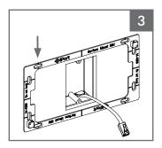
Install the (b) mounting bracket on the wall with the (b) bracket surrounding the electrical box. Use the centerlines as a guide to install the (d) mounting screws. Using the recommended screwdriver and mounting screws, install the first screw in the upper left hand corner.
