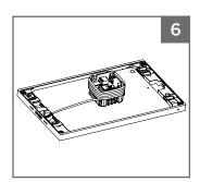
Connect the USB connector to the USB port located on the (f) PoE splitter. Tightly wrap the remaining iPad cable around the (f) PoE splitter.
