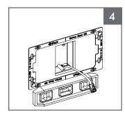
Level the (b) mounting bracket over wiring location and fasten (b) bracket with the remaining (d) screws using a Phillips screwdriver.
