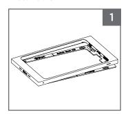
To decouple the (a) bezel from the (b) mounting bracket, place the (a) bezel face up on a flat and smooth surface. With one hand, hold the (b) mounting bracket in place. With your opposite hand, lift the right edge of (a) bezel and then the left to decouple the magnets.
