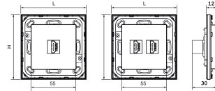
Mounting with frame: 81 x 77 (L x H) Mounting without frame ('NF): 80 x 80 (L x H)
