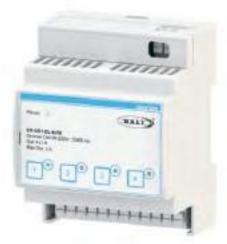
The 4-channel DALI-2 dimmer allows brightness control of LED and halogen sources with voltage 90-230 Vac 50/60Hz for up to 200Watts on 4 channels each. Input Bus DALI-2 reference IEC 62386 standard.
