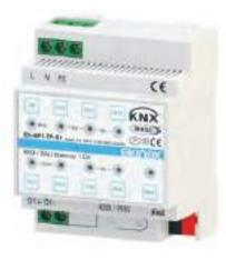
Ekinex® Gateways EK-BF1-TP-D1 is a device used to control electronic control gear (ECG) with a DALI interface (according to EN 62386) via the KNX installation bus. The device converts switching and dimming commands from the connected KNX system into DALI telegrams and status information from the DALI bus into KNX telegrams.
