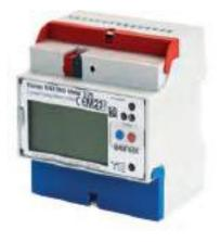
Three-phase MID energy meter for active and reactive energy measurement with bidirectional metering for imported and exported energy, current (A), voltage (V), active power (kW), reactive power (kVAr), power factor and other electrical parameters. Direct connection up to 75 A. The device has an integrated communication module to the KNX bus.
