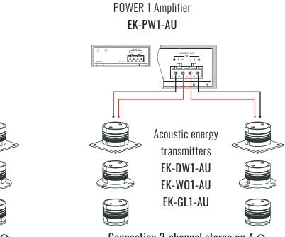
Connection 2-channel stereo on 4  $\Omega$ . Single transmitter applied power: 80 W
