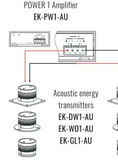
Series connection 1 mono channel on 8  $\Omega$ . Single transmitter applied power: 80 W
