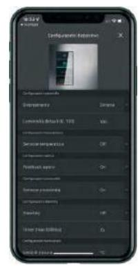
EKINEX TOOL" APP CONFIGURATION Settings page From the settings page, the main operating parameters of the device can be configured: display brightness, sensor enablement haptic feedback and stand-by time.
