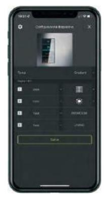
EKINEX TOOL" APP CONFIGURATION Pushbutton customisation page With a horizontal swipe you can scroll between the screens of the device and customise the related pushbuttons.
