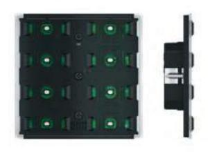
The 4-fold pushbutton of Ekinex® FF series commands loads on/off switching, controls the dimming of lighting devices, controls motor drives for shutters or executes any other programmable command and control function. The device integrates a KNX bus communication module and is intended for mounting onto a wall mounting box; it is supplied by a SELV voltage directly from the KNX bus and does not require any auxiliary power supply.
