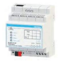
The Ekinex<sup>®</sup> M-Bus - KNX Gateway performs a protocol conversion between an M-Bus and a KNX TP network. The device acts as M-Bus master. Versions for networks with a maximum number of 20, 40, 80 and 160 connected M-Bus slave devices are available. The device integrates a KNX bus communication module and it is suitable for mounting on a 35 mm DIN rail; it requires an auxiliary power supply.
