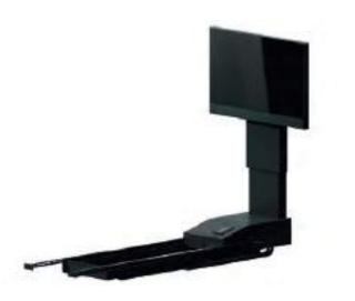
The EK-BTV-BL TV lift is designed and constructed to move a TV set under the bed. The product in the resting state is placed under the bed; by operating a wired control, the sliding motorised lift brings the TV set into the in-use state. The transition between the two states of rest/use takes place by means of three movements actuated by three electric motors:
