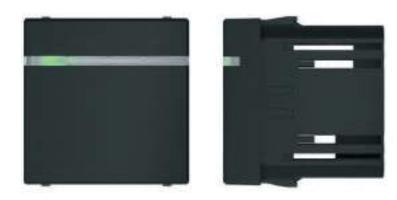
The Ekinex® EK-TR2-TP card reader with RFID technology is used for access control in combination with the EK-TH2-TP card holder pocket. Equipped with a bi-stable relay (4A@24Vac/dc), an input for potential-free contacts and a 3-colour front signal LED (white, green and red). The device has an integrated KNX bus communication module and is designed for wall mounting in a flush-mounted box; it is supplied with SELV voltage via the KNX bus and requires an auxiliary power supply at 12-24 Vac/dc.
