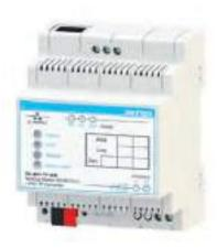
The Ekinex® Modbus RS485 - KNX Gateway performs a protocol conversion between a serial RS485 Modbus RTU and a KNX TP network. The device works as Modbus master. The device integrates a KNX bus communication module and it is suitable for mounting on a 35 mm DIN rail; it requires an auxiliary power supply.
