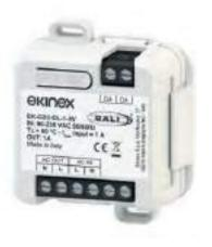
The single-channel phase cut dimmer EK-GD2-DL-1-HV allows the brightness control of LED and halogen sources with a voltage of 90-230 Vac 50/60Hz for up to 220Watts. Input Bus DALI-2 reference IEC 62386 standard.
