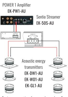
Series connection 1 mono channel on 8  $\Omega$ . Single transmitter applied power: 80 W
