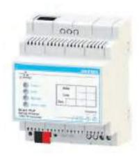
The Ekinex® BACnet - KNX Gateway performs a protocol conversion between a BACnet and a KNX TP network. Two versions are available: BACnet MS/TP (masterslave / token-passed) over serial RS485 network and BACnet IP over Ethernet. The device integrates a KNX bus communication module and it is suitable for mounting on a 35 mm DIN rail; it requires an auxiliary power supply.
