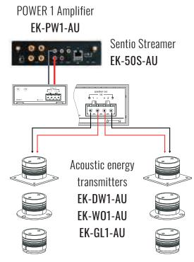
Connection 2-channel stereo on 4  $\Omega$ . Single transmitter applied power: 80 W
