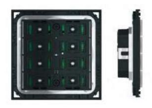
The 4-fold pushbutton of Ekinex® 71 series commands loads on/off switching, controls the dimming of lighting devices, controls motor drives for shutters or executes any other programmable command and control function. The device integrates a KNX bus communication module and is intended for mounting onto a wall mounting box; it is supplied by a SELV voltage directly from the KNX bus and does not require any auxiliary power supply.
