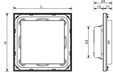
Mounting with frame: 81 x 77 (L x H) Mounting without frame ('NF): 80 x 80 (L x H)
