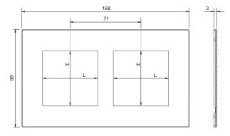
Adapter for Surface double plate WALL-MOUNT DEVICES
