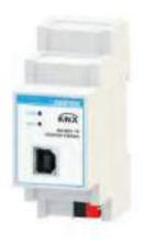
The Ekinex<sup>®</sup> USB interface EK-BD1-TP allows a bidirectional data connection between a PC and a KNX bus system. The device handles the addressing, parameter setting, display, protocol management and diagnosis of KNX bus devices. The device integrates a KNX bus communication module and is realized for mounting on a standard 35 mm DIN-rail.
