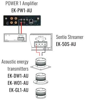
Connection 1 mono channel on 4  $\Omega$ . Single transmitter applied power: 200 W
