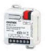
The EK-MS2-TP-TA device has 2 independent measurement channels via external current transformers (CT) and is suitable for measuring single-phase power lines (230 Vac, 50-60 Hz). The flush-mounted box mounting is made in a compact case with the possibility of mounting on a 35 mm DIN rail (EN 60715) using a special adapter included in the supply.
