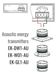
Connection 1 mono channel on 4  $\Omega$ . Single transmitter applied power: 200 W
