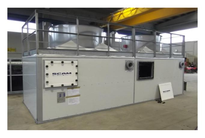
The *TAS / TASF SERIES* are dedicated to every industrial sector with a modular conception. These models are characterized by SCAM T.P.E. S.r.I. well defined standards and are supplied with a preassembled structure in hot galvanized steel according to EN ISO 1461 standard. The *TAS / TASF SERIES* are equipped with sandwich insulated walls (22-26 mm thick) made of expanded polymer covered by FRP, which guarantees an excellent aesthetics and a higher durability.
