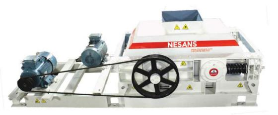
The double roll crusher CI Series is mainly used for Tertiary and Quaternary crushing of middle-sized materials. One benefit of the Nesans double roll crusher is the ability to produce a narrow particle size distribution, thus minimizing the production of undesired product sizes. The smooth roll crusher CI Series offers a suitable solution for fine grinding processes.
