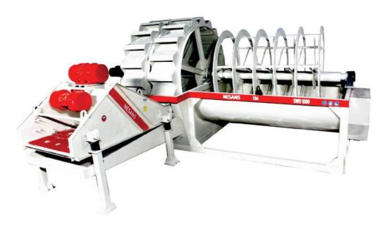
Nesans SW D Series are bucket classifiers with Dewatering Screen complete with fines retention screw, bucket wheel fitted with PU panels for the removal of clays, silts and slimes to produce up to 2 grades of sand. The SW D Series is designed to operate with maximum versatility and can support different requirements such as maximum retention of fines or maximum disposal of fines.
