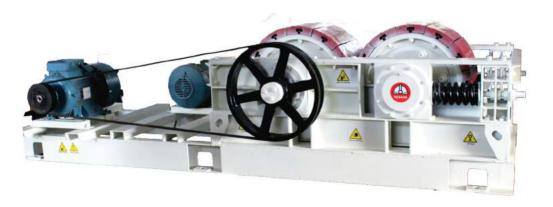
The roller shells are made of highly wear-resistant cast alloys. The possible efficiency is between 60 and 70 per cent of the cover thickness. In order to facilitate maintenance, the smooth roller shafts are arranged in labyrinth-sealed plummer blocks with lubricated, amply dimensioned spherical roller bearings.
