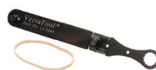
3044 VERSATOOL™ Locates holes as well as starts and tightens hex nuts onto rail bolts. Drives 5/16" rail bolts and tightens 1/2" hex nuts. Also used to locate 1/4" pilot hole on handrails & rail drops for attaching to Connect-A-Kit® handrail fittings.
