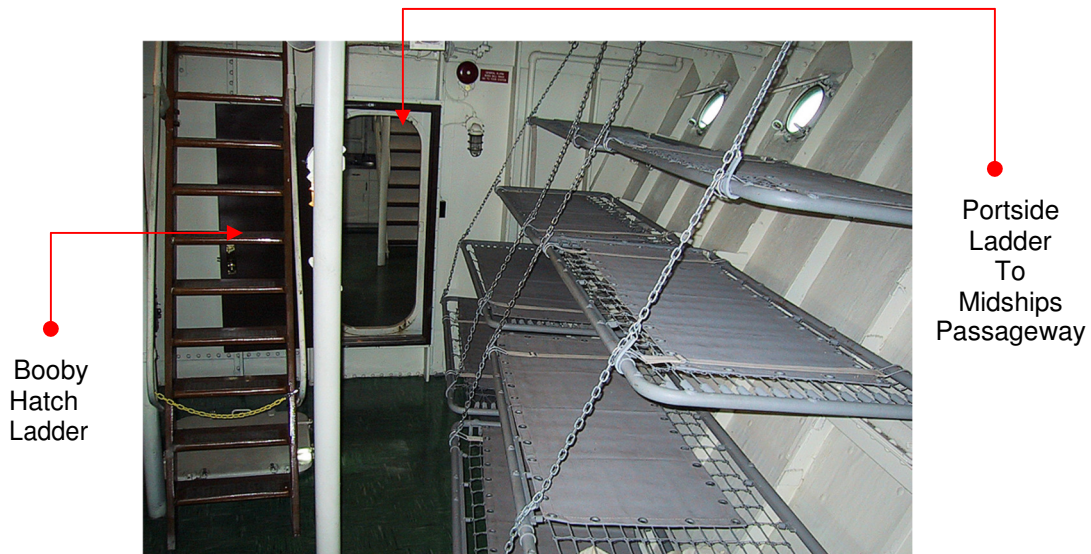
Figure 25 – Crew's Quarters; Forward Compartment
