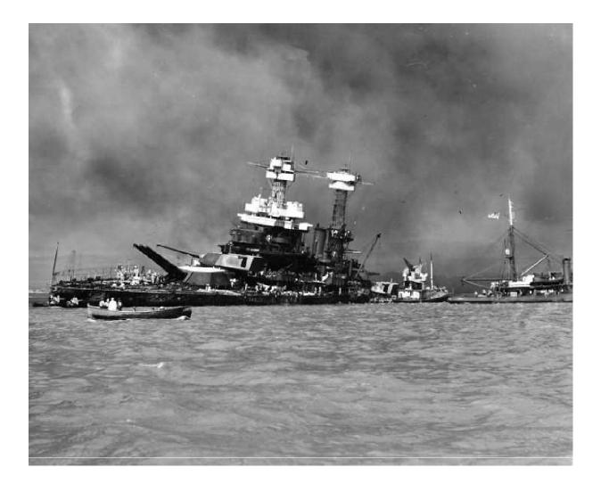
In the second Japanese attack wave the California also suffered from an explosion by a bomb that penetrated to the second deck. The explosion caused the rupture of the forward bulkheads as well as intensive fires.
