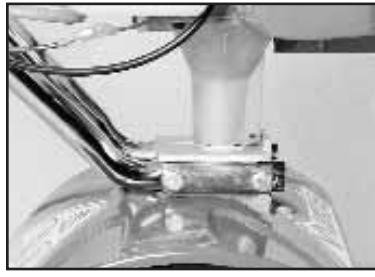
Picture 2 ... Note how the engine sits all the way down on the transmission.
